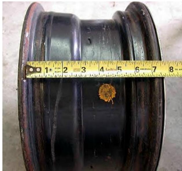
A common mistake when measuring a rim's width is measuring the absolute width of the wheel.
